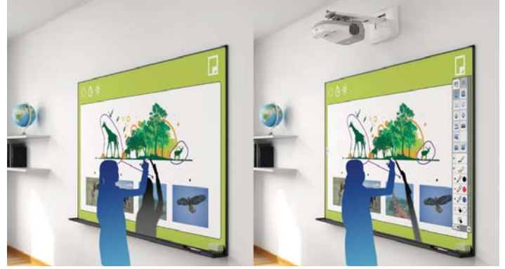
Conventional projector with shadow interference
